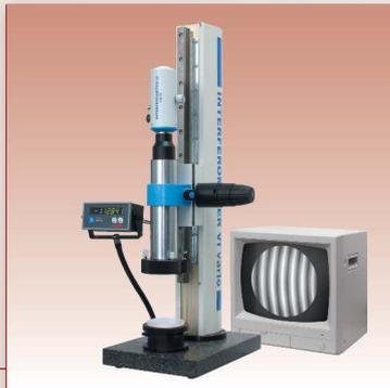
Workstation for testing of prism surfaces.
