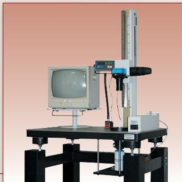
Workstation for quick testing of small plane optical components.
